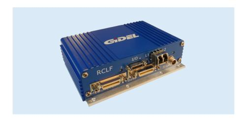
The Remote Camera Link Fiber-Optic (RCLF) extension system enables frame acquisition from a remote camera at a distance of up to 40 km without repeaters. A remote camera connects directly to the RCLF module that transmits the camera image over fiber optic cables to either a Gidel PCle HawkEye-CL frame grabber board mounted in a host computer or to another Gidel RCLGR module that can interface with any user frame grabber.
