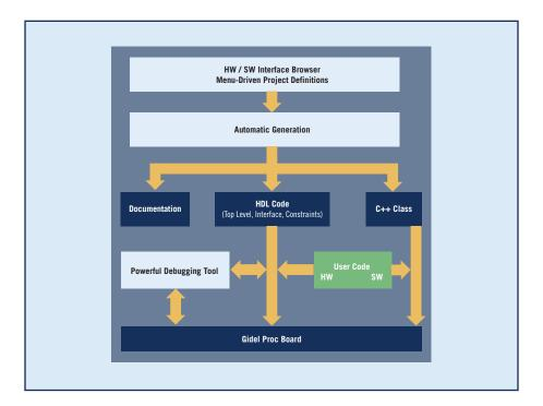
Gidel's developer's suite provides a powerful set of tools and a methodology for simplifying the development task and reducing development time. The suite includes the following components:
